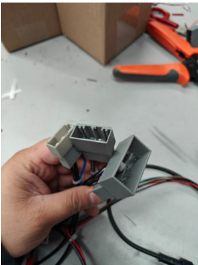
car side connectors plug into factory plugs
